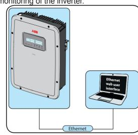
When the inverter is connected to the LAN network with access to the Internet, the Ethernet board allows to transfer data to the Plant Viewer/Aurora Vision® portal for remote monitoring purposes (over an Internet browser)
