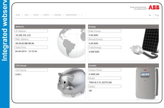
The **HOME** screen shows general information about the network (IP address, MAC address, date and time), the generated energy, the CO2 emissions and the inverter (output power, inverter model and inverter state).
