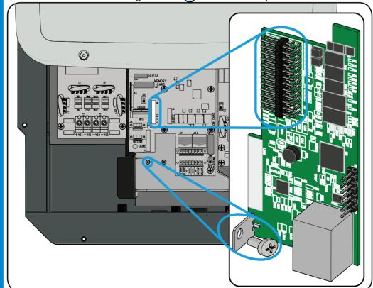
Once the installation is completed, the Ethernet cable can be connected to the dedicated port.
